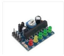
KA2284 Power Level Indicator Battery Indicator Pro Audio Indicating Module 5Y
